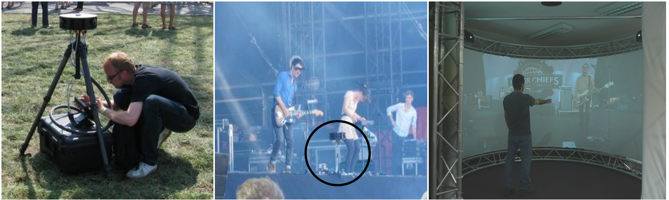
Figure 1. ODV workflow. From left to right, an omni-directional camera, the recording process during a concert, and projection of the resulting omni-directional video in a CAVE-like setup.
